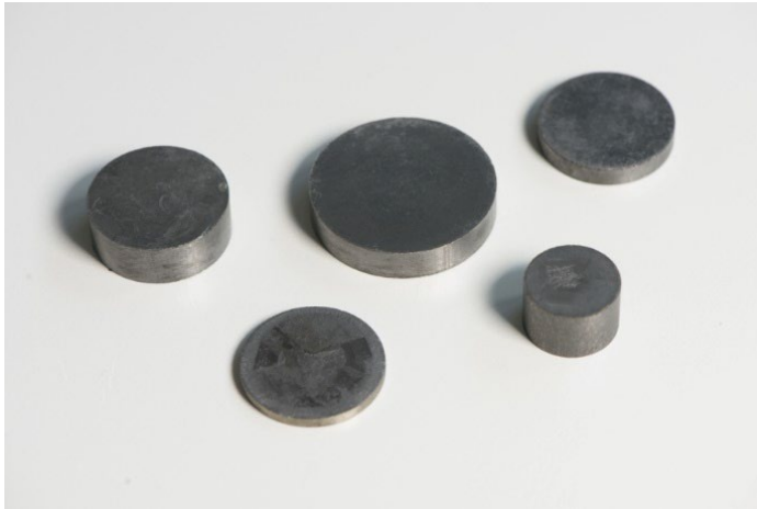
Fig. 2: Magnet production: The magnets contain a mixture of neodymium as a primary raw material and recycled magnets or magnetic scrap. This makes it possible to reduce use of valuable raw materials.
