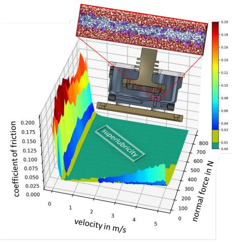
Application-oriented demonstration of superlubricity between two oxidized silicon carbide surfaces by means of slide-pad tribometer and molecular dynamics simulations (blue: water; violet: dissolved ions) (© Fraunhofer Institute for Mechanics of Materials IWM).
