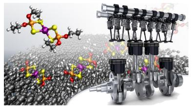
The ZDDP molecule from the lubricant additive (colored) is triturated between the ta-C layers (gray). Sulfur atoms are rubbed into the diamond-like carbon layer and weaken it. Right: Application example combustion engine. (© Fraunhofer Institute for Mechanics of Materials IWM)
