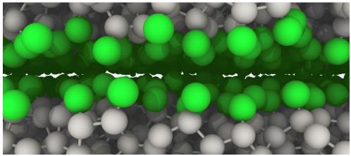
Tribological contact of two fluorine-terminated DLC surfaces (carbon grey). The (green) fluorine terminations can become "obstacles" upon sliding and increase friction. (© Fraunhofer Institute for Mechanics of Materials IWM)
