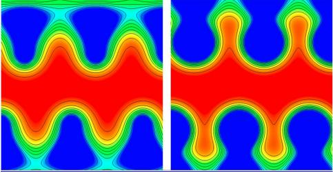
Electron density of two hydrogen-terminated (left) and fluorine-terminated (right) diamond surfaces: large fluorine atoms prevent the surfaces from interlocking and thus reduce friction.
