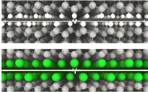
Tribological contact of two hydrogen (top, white) and fluorine-terminated (bottom, green) diamond surfaces (grey): fluorine passivation halves friction compared to hydrogen passivation.
