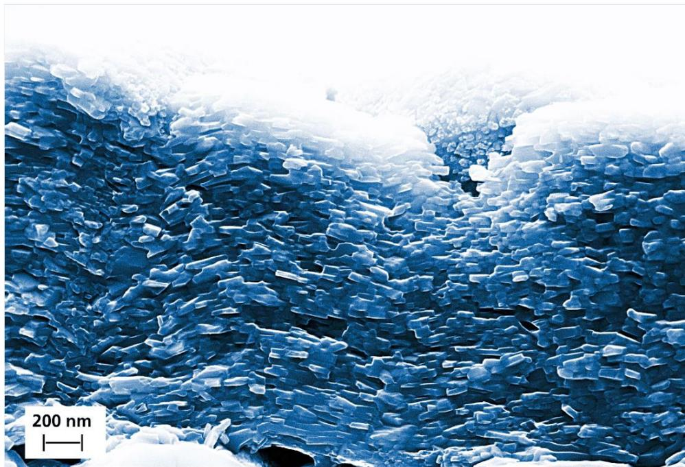
Fig. 1: REM image of the fracture edge of a Ti<sub>2</sub>AlN coating with platelet-like shaped grains.
