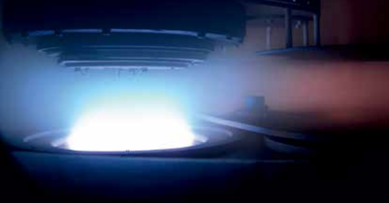
View into a high-frequency magnetron system (coatings for glass soldering).
