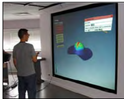
Figure 3. Application of the VR in the study of the Nakazima FE simulations: study of the localized necking and the failure.
