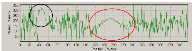
Figure 10: Graph of the linescan. The phase shift on the left side (marked black) occurs from the electrical contact, the phase shift marked red comes from the defect.
